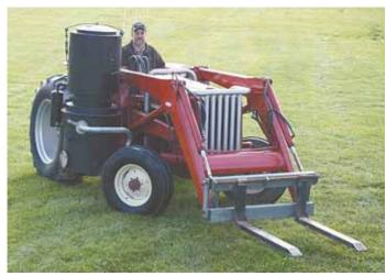
Ron Lemler's wood gas-powered tractor runs on wood scraps from his pallet factory. Last spring the 1978 IH 574 tractor powered a 4-ft. tiller.
