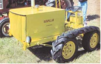
Layman Cornelison's "Ratapiller" is powered by a 1980 Chevette engine. Tracks were made from the rear tires off a Farmall C tractor.
