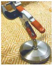
"The stand uses a spring-loaded clamp to hold the micrometer. It works like a third hand. I riveted one side of the clamp to a curved 1/2-in. dia. bolt, which screws into a nut welded on top of a 4-in. dia., 3/4-in. thick round metal base."
