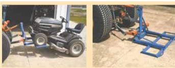
Home-built, 3-pt. mounted service lift lets Jerome Webb work under his riding mower without removing the deck. A pair of square lift frames support mower's front wheels.
