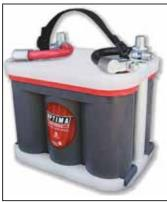
Custom CNC-machined battery pack in-cludes a pair of Optima 6-volt AGM Red Top batteries harnessed together in parallel. They provide 2,000 cranking amps of 6-volt power.
