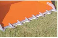
Loader bucket-mounted Piranha tooth bar works great to clear brush and rake out roots.
