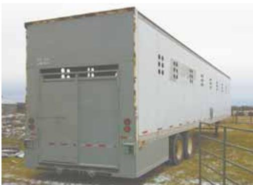
Gary Bueckert saved the cost of a new cattle hauler by converting a semi trailer into this ground loading model. The former 53-ft. van carries about 30 head at a time.
