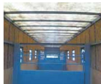
He lowered the last 7 ft. of the van to build a ramp and also installed an endgate. Photo at right shows stalls inside trailer.
