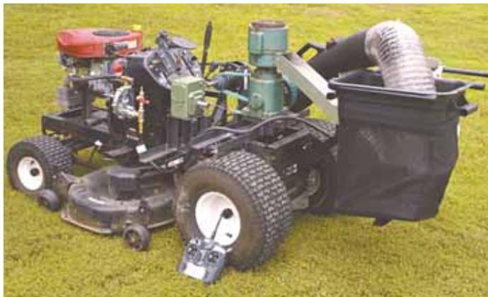
Remote-controlled, garden tractor-sized mower pelletizes grass clippings and then feeds the pellets into a burner that powers the machine.
