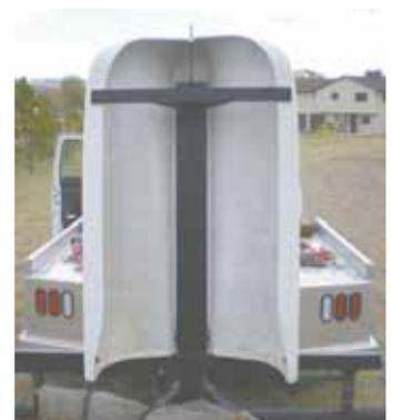
Dale Hiatt made this trailer-mounted bug deflector by bolting together 2 air deflector side panels off a semi truck. Deflectors are supported on back by an angle iron frame.
