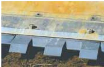
both a standard edge and a toothbar. I can grade, dig, level and back drag with no need to change-out. It has a specially designed serrated edge with flush-mounted teeth, so it'll dig into difficult terrain that standard edges can't handle. It works great to break up hard, dry clay and was almost like adding 20 hp and 2,000 lbs. to the skid loader, compared to when I used the bucket's original straight edge.
