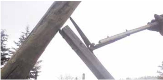
Luke DeWit used a pair of old barn hinges, a hockey stick, and a 6-ft. long 2 by 4 to make a jack that he uses to straighten wooden fence posts.
