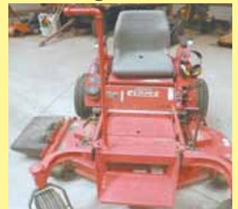
Pipe "assist handle" bolts onto deck of zero-turn mower.
