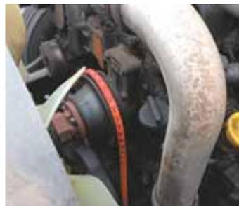
tow truck towed to a shop ([www.grainger.com](http://www.grainger.com); ph 800 472-4643). The A/C clutch froze on the wrecker, and no one in our area had a 'bypass' belt in stock. Once we installed the Power Twist belt we were able to drive the truck back to the shop for repairs."
