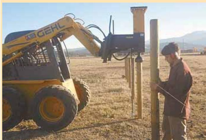
Floyd Yoder's skid loader-mounted fence post driver works fast, hammering posts like a jackhammer at 800 pneumatic blows per min.
