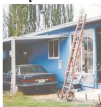
When the ladder is up against a building, the wheels are off the ground.
