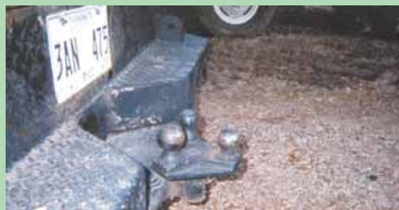
Rotating tri-ball hitch comes with 3 hitch balls in 7/8, 2, and 2 5/16-in. sizes that are welded to a steel plate.
