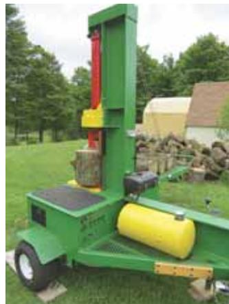
A pair of push buttons are used to operate the loading arm, and a control lever operates unit's 2-stage splitting wedge.
