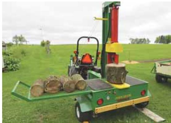
A 12-volt winch is used to raise and lower the 5-ft. long loading arm on Ed Hollmer's vertical splitter. "Very little lifting or bending is required," he says.
