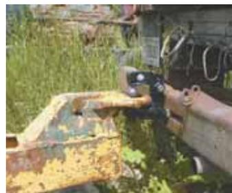
Dean Konsela came up with an adapter for the DMI hitch on his pickup, allowing him to safely pull a pintle hitch trailer.
