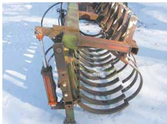
He used 4 by 2 tubing off an old cultivator to build the frame, which supports 2 rows of spring-loaded shanks spaced about 7 in. apart.
