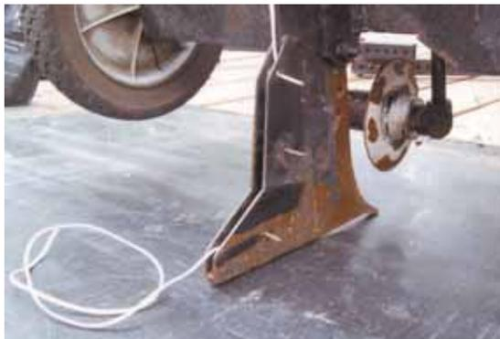
Cal Miner built this 2-wheeled “mini plow” so a friend could install underground invisible dog fencing around his 3-acre yard.
