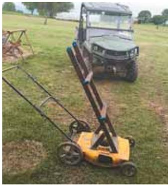
“Feed bucket carrier” is bolted to mower deck and looks like a short ladder tilted backward. It holds up to three 5-gal. buckets.
