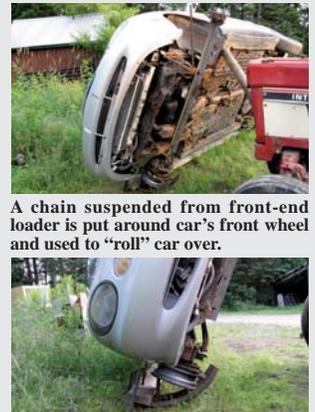
He first takes the wheels off one side of car and then attaches roll bar brackets – pieces of curved pipe – to both hubs.
