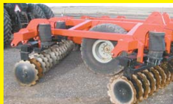
Field Disk Controlled By Air Bags (Page 2)
