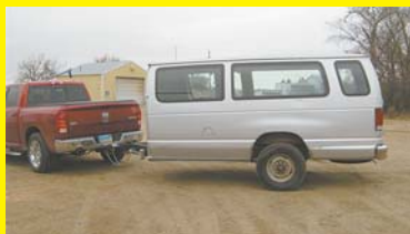
Enclosed Trailer Made From Old Van (Page 33)
