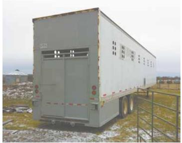
Gary Bueckert saved the cost of a new cattle hauler by converting a semi trailer into this ground loading model. The former 53-ft. van carries about 30 head at a time.
