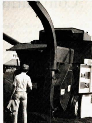
Purdue-built attachment saves 80% of the cobs that pass through the machine.
