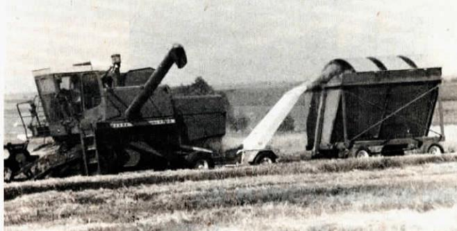
Besler residue blower is powered by a 16 hp. gasoline engine.
