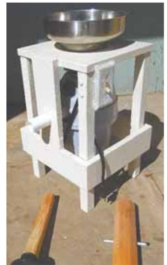
Electric-operated garbage disposal mounts inside wooden stand. Bowl with hole cut into the bottom funnels apples into disposal.
