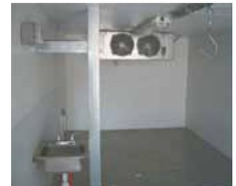
Knott's truck has hot water to wash down carcasses, a track to hang up to 3 cows or 40 pigs at a time, and a refrigeration system to cool the meat as he hauls it back to his processing facility.
