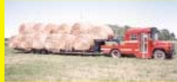
drawer toolbox is bolted to the bottom side of the bench. We cut off the last two feet of the bus and, with the help of a couple of neighbors, moved this 2-ft. section forward and then welded it onto the back of the front section. We bolted a steel plate on back for pulling a fifth wheel trailer and wired it for lights. We also painted the bus Case-IH red and added two white strips. (**Larry Rodgers, Box 14, Lavenham, Manitoba, Canada R0H 0P0 ph 204 252-2120**)
