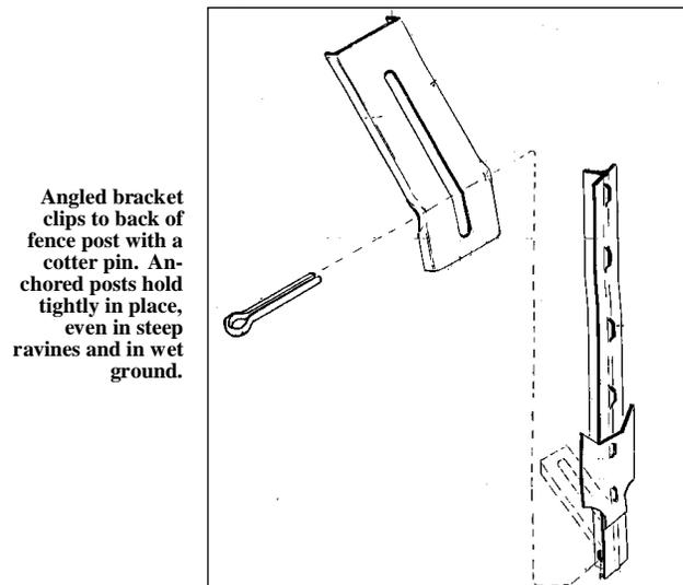
Angled bracket clips to back of fence post with a cotter pin. Anchored posts hold tightly in place, even in steep ravines and in wet ground.
