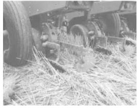
HCS furrow-closing wheels replace the original closing wheel with two independent arms, each holding a spoked wheel.
