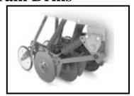
Worn depth control assemblies show three points of wear - side plates; steel bushings and adjustable pin; and press wheel adjust-
