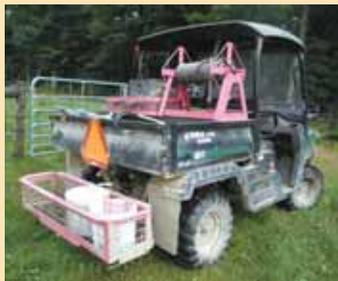
Wilson also built a rear rack for his wife using angle iron on a base frame of 2 by 2-in. tubing that fits the UTV receiver hitch. It holds 5-gal. pails for hauling supplements.
