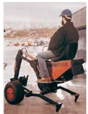
Small enough to fit through a garden gate, this 2-wheeled mini excavator has a 5-ft. long reach and can dig down about 4 1/2 ft.
