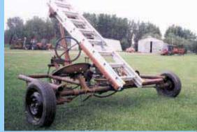
This self-propelled ladder moves around the farm at speeds up to 6 mph. "It's very stable. You don't have to worry about the ladder kicking out or the wind blowing it over," says the Alberta inventor. See story on page 2.
