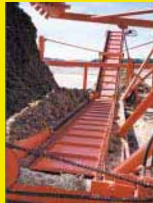
Shaft that rolls up plastic is positioned above conveyor so all remaining silage drops onto conveyor as plastic is rolled up.
