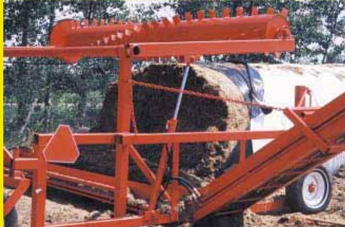
Large tooth roller peels silage off end of bag, dropping it onto paddle conveyor that carries it to a feed truck or wagon. Unloader is pulled ahead by rollers that roll up plastic.
