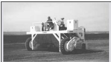
Scarab's new self-propelled turner is designed for smaller operations. It's competitive with pull-type machines because tractor isn't needed, the company says.
