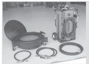
Oil Transfer system lets you filter new oil before it goes in and also "repurifies" used hydr aulic oil back to original specs so it can be reused.
