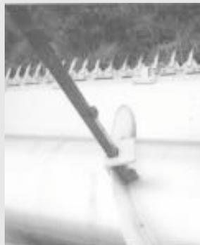
**To straighten out a bend, Lassila sets 4-ft. long bar on side of auger flighting away from the bend and slides angle iron piece down over flighting.**
