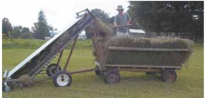
**Gies bought an 18-ft. long, 4-ft. wide hay loader, reversed the belt direction, and mounted it in front of a wagon. He mows, rakes and loads 6 acres of hay 3 times every summer.**
