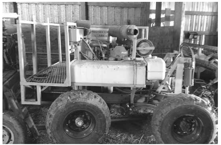
Forecart is equipped with a 115 hp, 3.9-liter turbocharged Cummins diesel engine, mounted on 1-ton Ford truck axles butt-welded together.
