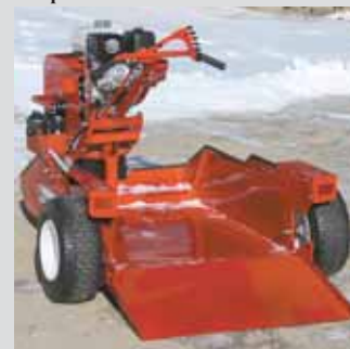
Powerhouse Wheelchair Driver allows Marvin Kauffman quick access to the yard and office where he works. Tailgate ramp is used to roll chair into driver's compartment.
