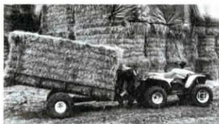
is easier to use than most bale transport trailers since it rides so low to the ground and the ATV is easy to get on and off. The trailer is 8 1/2 ft. long, 4 1/2 ft. wide and has low siderails that help hold bales in place. Can also be used to haul small square bales. We're looking for a North American distributor. Sells in Britain for about \$1,000. (M.K. Engineering, Unit 1, Hawkers Farm, Dores Lane, Braishfield, Romsey, Hampshire SO51 0QJ England ph 0794 68695; fax 0794 68537)
