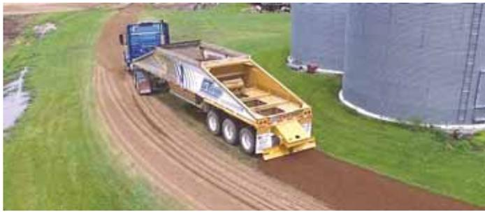
The new GT II Spreader attachment for belly dump trailers is shown here spreading gravel at about 10 mph around some grain bins.
