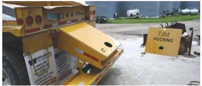
Spreader replaces belly dump trailer's existing push block with an air-operated, 16-in. high steel blade just under 8 ft. wide.
