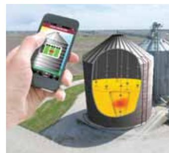
Phone and table app reads grain temperature through sensors inside bin and displays it visually on any device with internet access.
