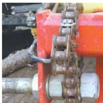
**Ross Dormire used pieces of roller chain to reinforce the connecting pins on both sides of the hitch on his 3-pt. mounted sprayer.**
