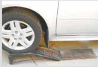
"This is just a handy hint. I have one car that's very low to the ground so when I drive up on the ramps, the front end rubs on the ramps. So now I lay a piece of 2 by 12 in front of each ramp to gain a bit of height before the wheels go onto the ramps."
