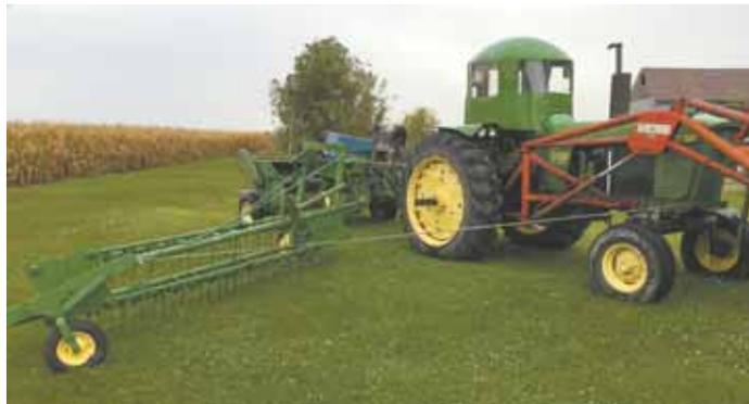
Home-built ditch rake brings mowed ditch hay into a windrow on side of road for baling. It'll handle a 10-ft. swath.
