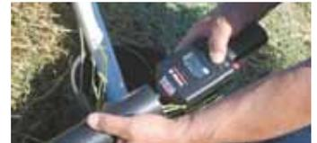
Electronic moisture readings are recorded from 4 levels in collection chamber and then averaged.
