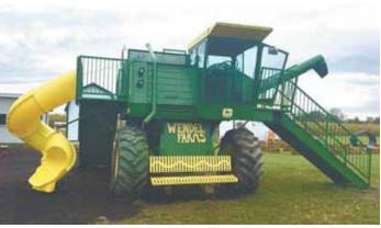
"Jungle gym" was built out of an old Deere 6600 combine. Two large stairways and platforms were added around the cab with a large slide on one side.
