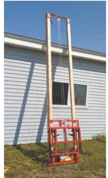
Rail Hoist uses a cable hoist at the bottom to operate a carriage that lifts loads up to 350 lbs.
