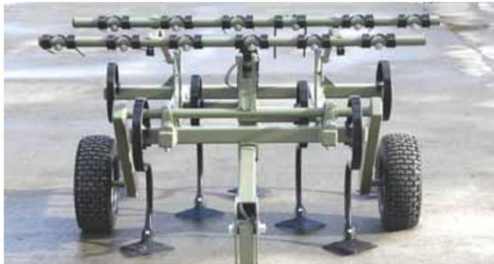
ATV-pulled cultivator is equipped with 3 rows of S-tines with 7-in. shovels and a 2-gang harrow on back. A 12-volt screw actuator controls shovel depth.
