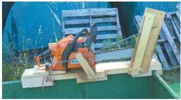
"Trigger rod" revs up chainsaw. It consists of a short rod that runs through chainsaw handle and under the trigger, and a longer "spring-loaded" rod that runs alongside chainsaw bar.
