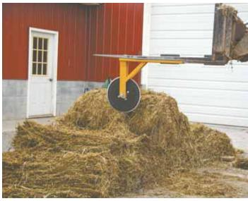
Sharpened coulter mounted on a tubular steel arm slides over skid loader fork. Down pressure alone is enough to slice through bales.
