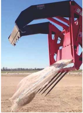
Loadermounted round bale splitter holds onto net wrap so you can release it in a convenient location and keep it out of your feed grinder.
