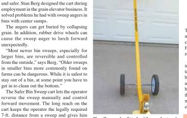
Handle can be fitted with an electronic control that has a dead man's switch (shown below).
