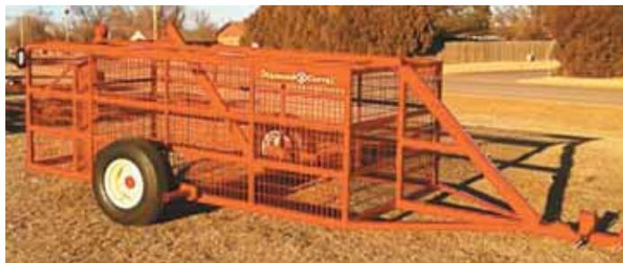
Trailer-style hog trap sets up in just a few minutes. A one-way gate keeps trapped hogs in while allowing hogs outside to push through gate and get trapped, too.
