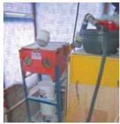
Andrew Sewell hooked up a shop vac to his 'gasblasting cabinet" to turn it from positive to negative pressure and stop it from leaking (above). A homemade bleed valve is used to regulate vacuum in the chamber.
