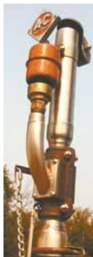
Justin Kelzer uses the exhaust from his D-17 Allis Chalmers diesel tractor to power a whistle that sounds like a train. A cast iron school bell mounts on front of tractor.
