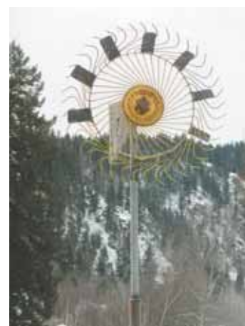
Windmill's metal blades are pop riveted to rake wheel's perimeter and set at a 15 degree angle to catch the wind.
