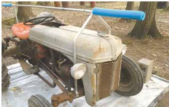
Pool noodles cut in half slip over front and back of frame to keep from tearing tarp.
