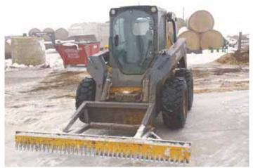
Dick Wise converted an 8-ft. grader blade into this scarifier with notched, sharpened teeth. Quick-tach 3-ft. extension improves visibility for driver.
