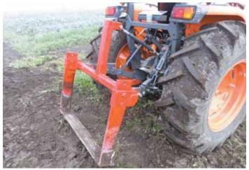
Bed Lifter blade passes under root crops, lifting and breaking up the packed soil to make harvesting easier.
