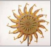
Ho-Bits fit over the teeth on a rotary hoe wheel and are welded in place with a jig the company provides.
